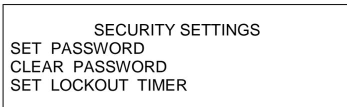
The Security Settings screen allows you to set a Control Panel menu password to prevent unauthorized changes to the power supply settings. After the Control Panel menu password is set, you will be prompted for the password when attempting to change the power supply settings.
