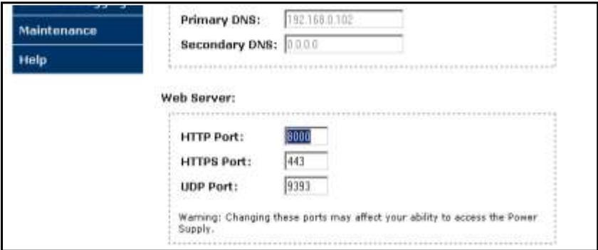
3. To configure HTTPS forwarding, repeat steps 2a – 2e with the HTTPS port number that the panel is using. If you are using the default panel port settings, the HTTPS port number is 443.
