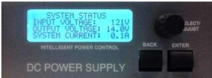
(Figure 2 Front Panel Display and Control)
